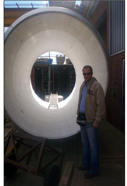
Ceramic fibre blanket rated up to 1420°C
